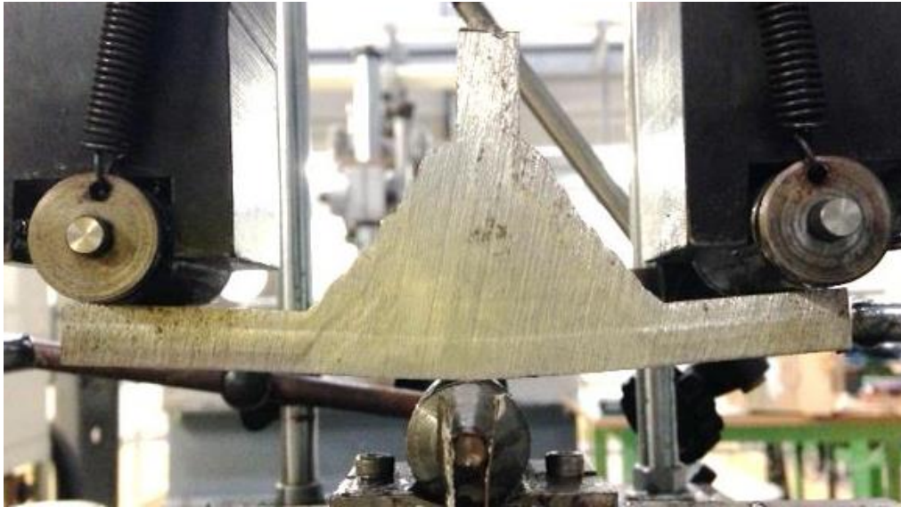
Fig. 4.11 Specimen's configurations of the fatigue test machine
