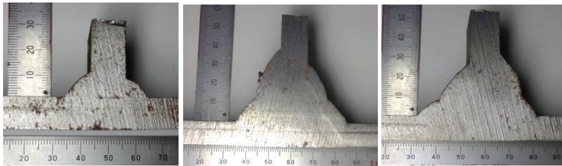
Fig. 4.1 Schematic illustration of welded specimen used
