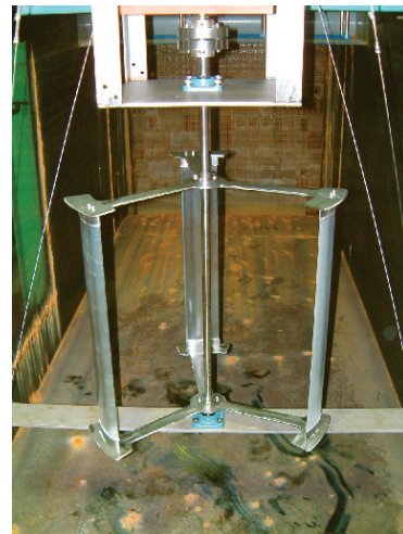
Fig.1 Experimental apparatus in the circulating water channel (B x D=1.5m x 1.2m)
