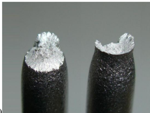
Fig. 3 Tensile test of SUH660 steel: (a) stress-strain curve; (b) fractured tensile specimen.
