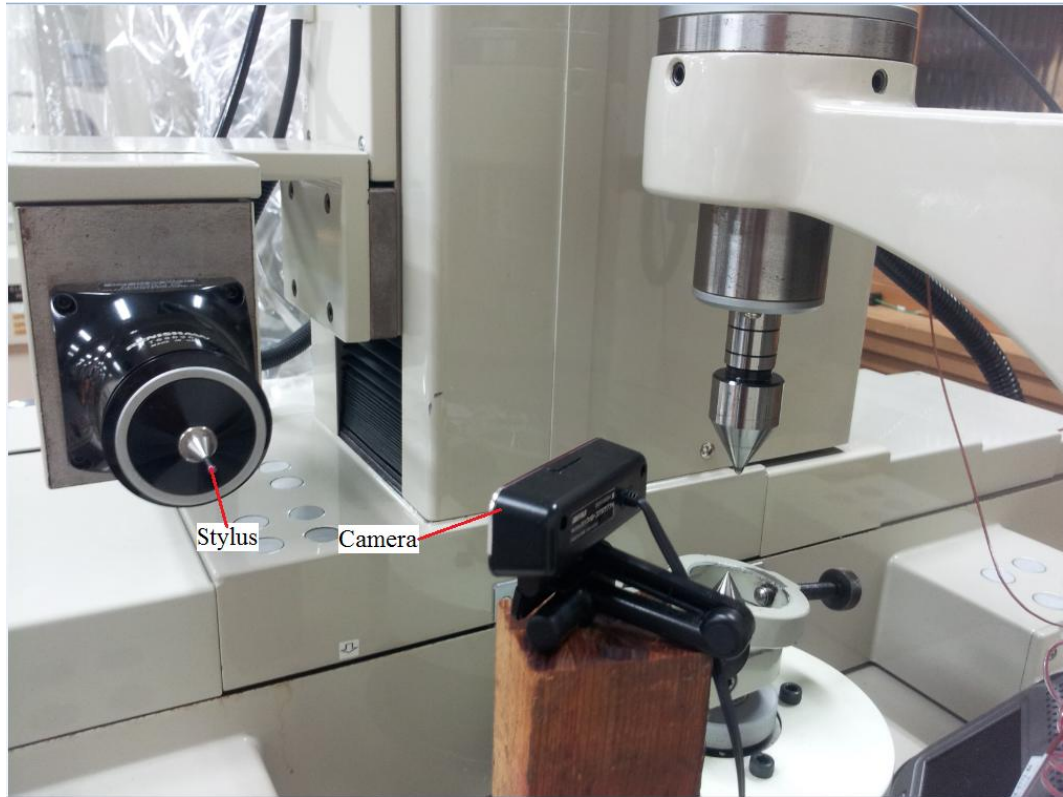
Fig. 4. 1 Camera setting to track the stylus
