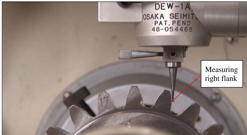
Fig. 3. 3 Conventional measurement: scanning of left tooth flank
