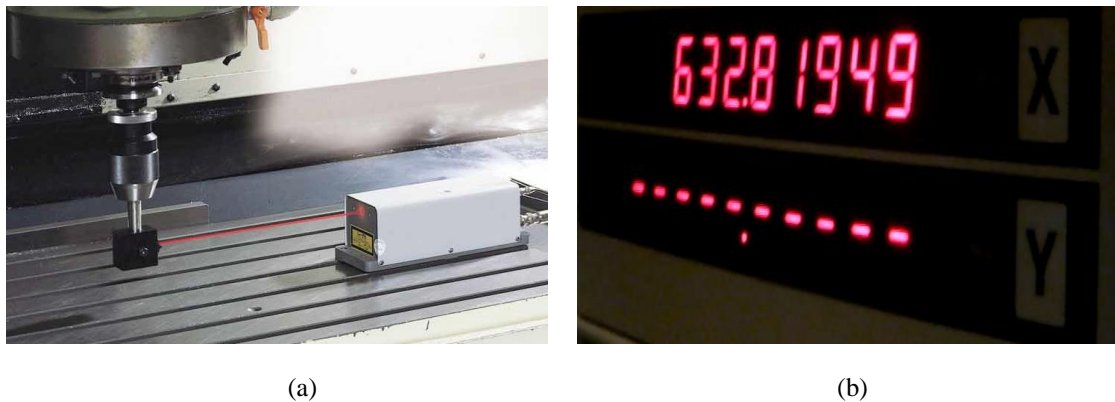
Fig. 3. 9 (a) An active laser interferometer during manufacturing process; (b) an example of correct laser beam radiation before measurement
