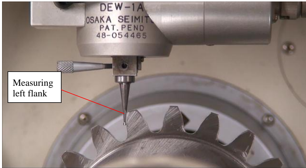
Fig. 3. 3 Conventional measurement: scanning of left tooth flank
