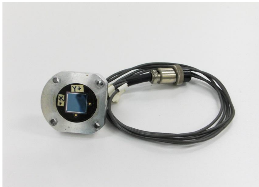
Fig. 3. 12 PSD sensor for front axis setting
