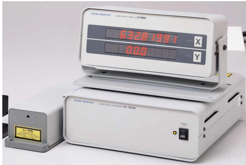
Fig. 4. 2 A set of complete laser interferometer
