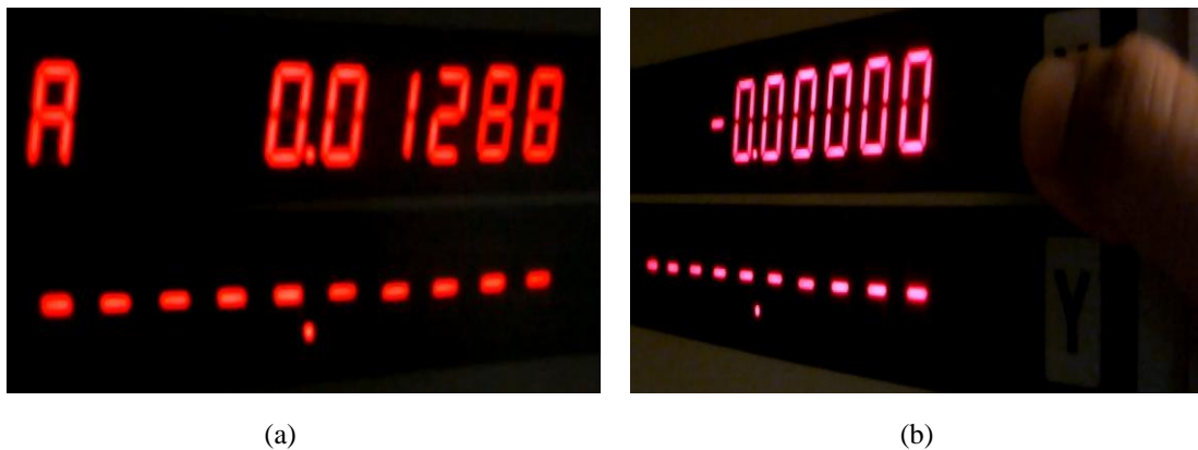
Fig. 3. 10 (a) An example of active measurement while generates alarm in monitor; (b) Laser interferometer monitor after resetting the button
