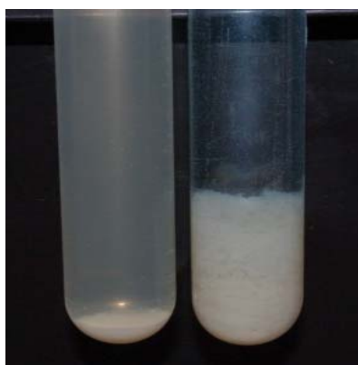
Fig.2.8 Phosphates can precipitate with \text{Ca}^{2+} without pH adjustment shown in the left test tube; nearly total phosphorus can be precipitated with \text{Ca}^{2+} at pH 11 shown in the right test tube
