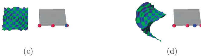
FIGURE 5. (c): the target shape matches the blended shape when the weights are (0, 0, 1) . (d): the weight can be outside the range of 0 to 1; this means extrapolation.
