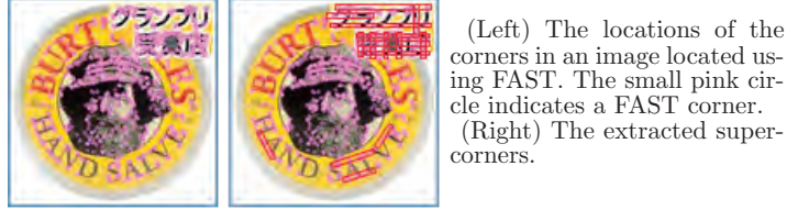
FIGURE 2. Extracted FAST and Supercorner
