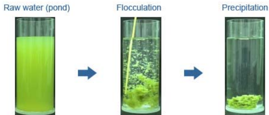
Fig.2.6. An Example of water sample treated by flocculation/coagulation process.
