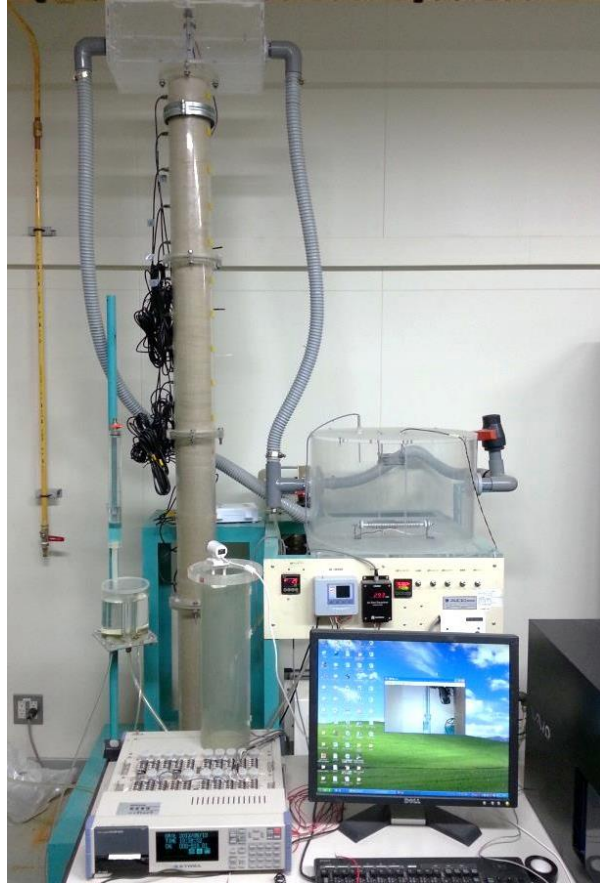
Figure 5.3 Picture of the setup of column evaporation test with constant water table
