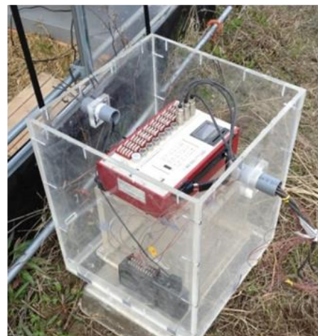
Figure 6.4 Photos of the lysimeter test, (a) thermocouple and water moisture probe, (b) soil column, (c) bird view of lysimeter, (d) data acquisition system, (e) final appearance
