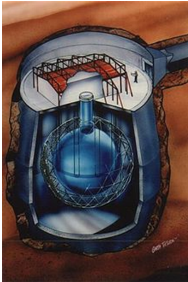
Figure 1.6 The concept of SNO's detector.
