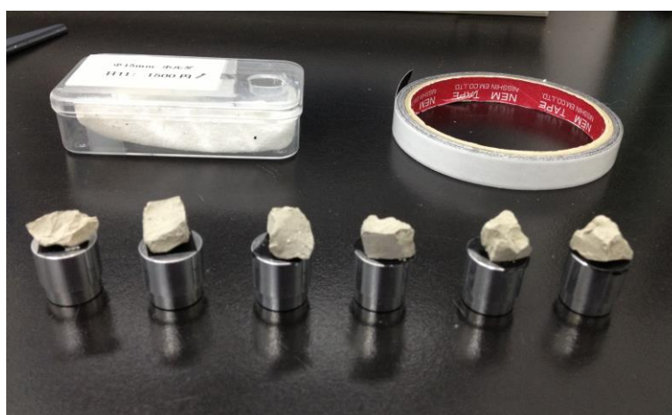
Figure 3.10 Preparation of scanning samples
