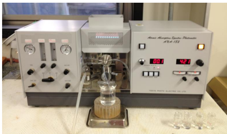
Figure 3.5 Atomic absorption spectrophotometer (ANA-182) apparatus
