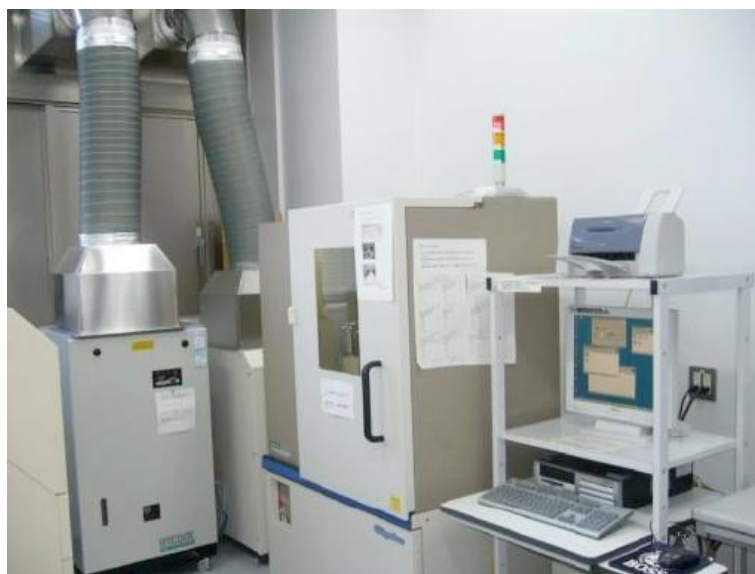
Figure 3.12 Automated Powder X-ray Diffractometer (MultiFlex)
