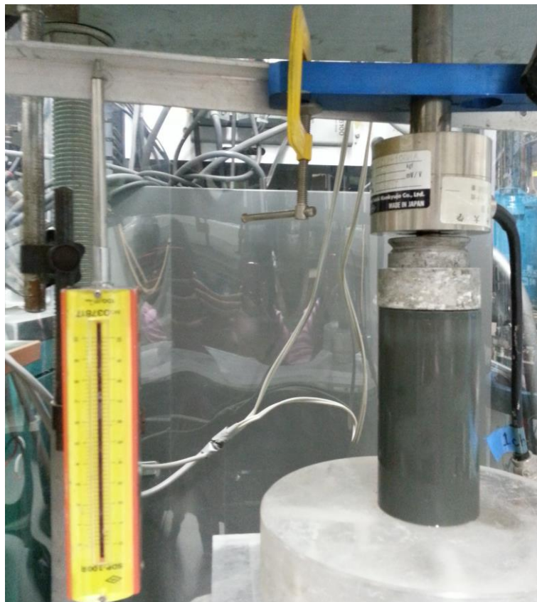
Figure 3.4 Unconfined compressive strength tests
