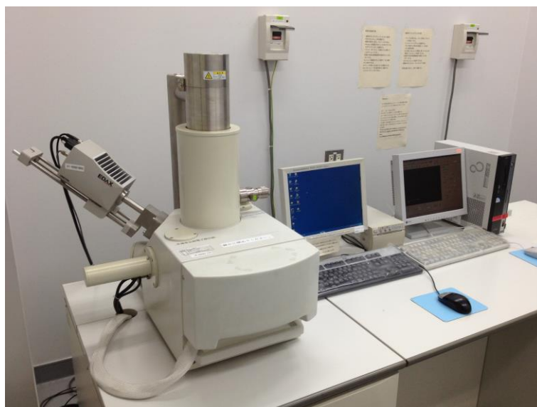
Figure 3.9 Scanning Electron Microscope (Super scan SS-550)
