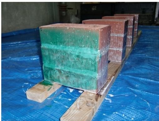
Figure 5.41 Application of adhesive
