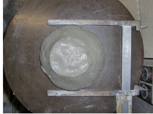
Figure 5.2 Flow test on ECC mortar
