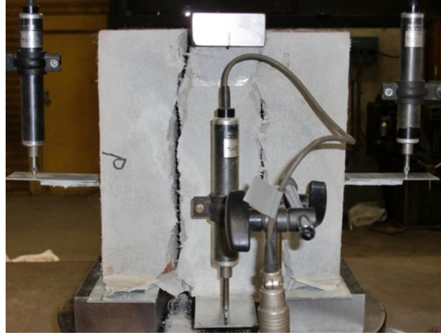
Figure 6.1 Crack propagation in ECC retrofitted triplet specimens
