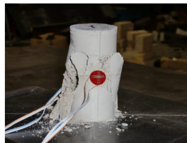
Figure 5.12 Compressive test on bed joint mortar
