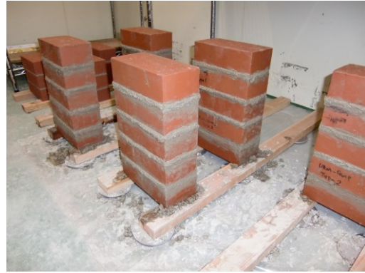
Figure 5.18 Construction of UP specimens
