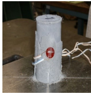
Figure 5.4 Compressive failure of ECC
