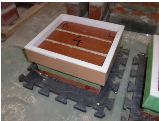
Figure 5.19 Molding of RT specimens
