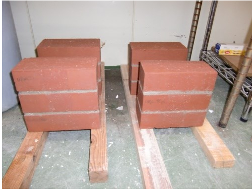
Figure 5.17 Construction of UT specimens
