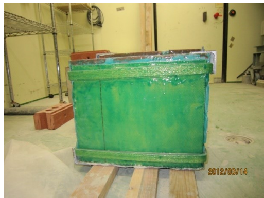
Figure 5.44 Wrapping confining bands
