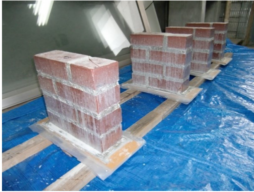
Figure 5.39 Application of primer
