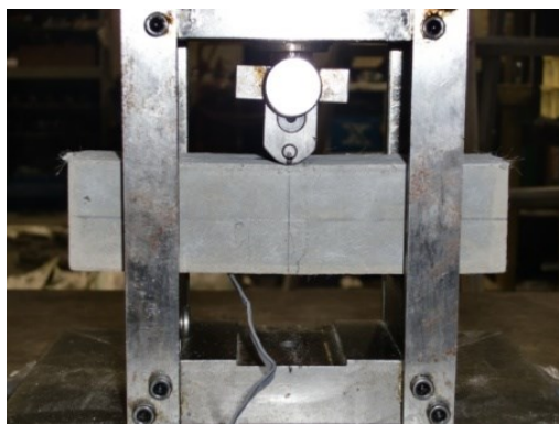
Figure 5.5 Bending test on ECC
