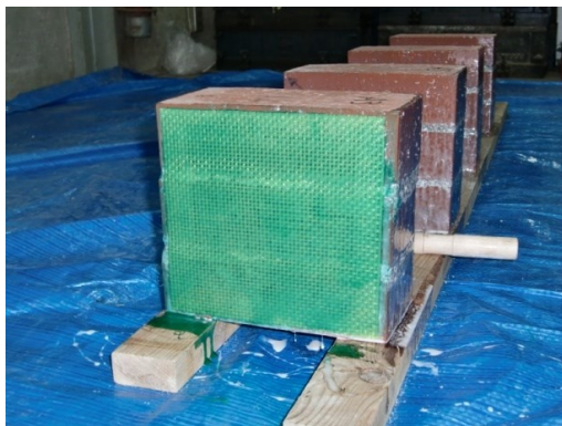
Figure 5.43 Coating with adhesive
