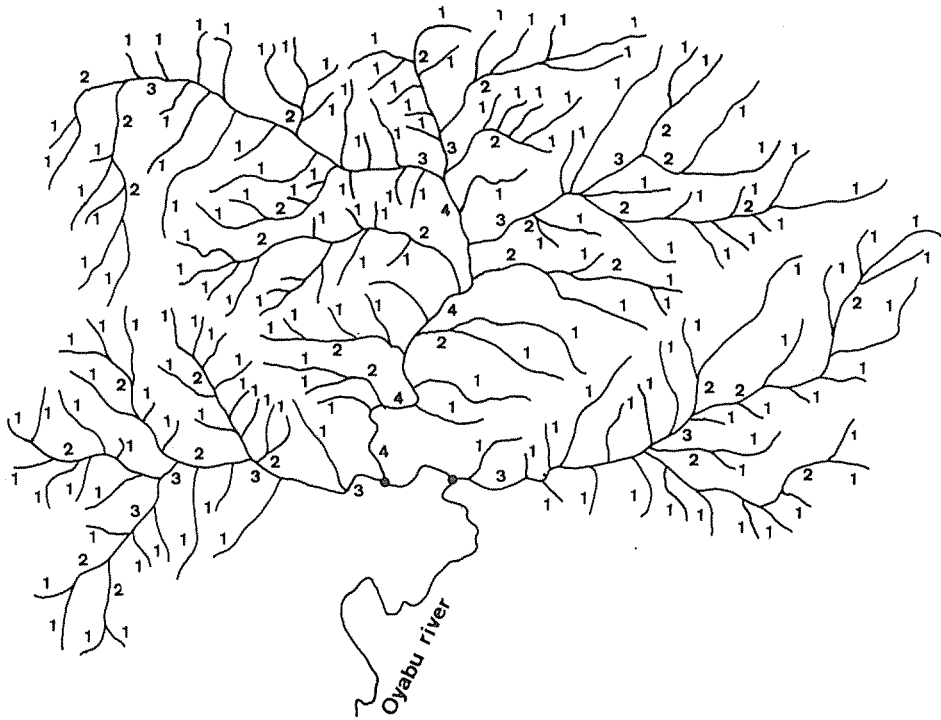
Fig. 4 Drainage network and stream order of the Oyabu river basin. 図4 大藪川の流路網と流路次数
