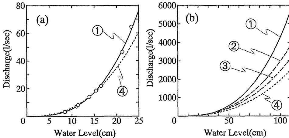
Fig. 4 Stage-discharge rating curves of the measuring flume.
