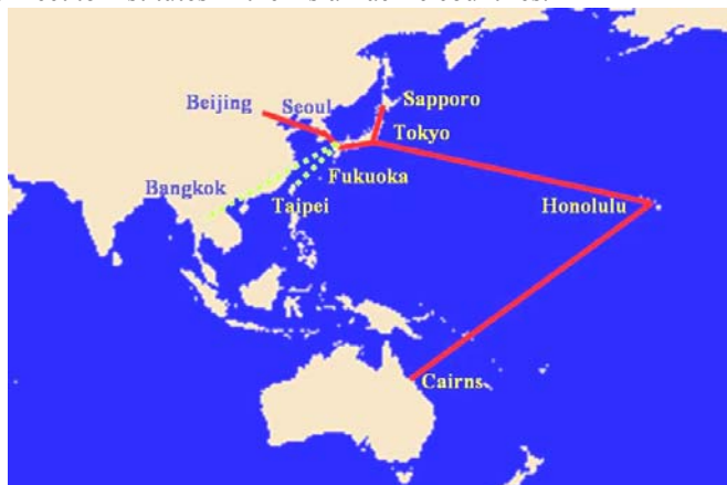
Figure 1 The network configuration in Asia Pacific area in the project. The solid lines show the network we have established, and the broken lines show the network we are planning to establish.
