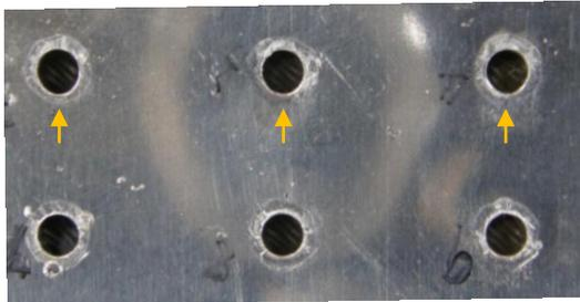
(h) bearing deformation of Al-patch fastener holes (c)
