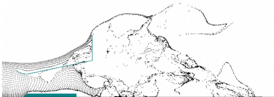
Figure 15: Instantaneous flow field for the simulation without wind turbine blades.
