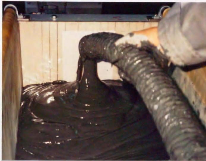
Photo. 6.5 Packing Ariake clay in slurry condition in soil bin
