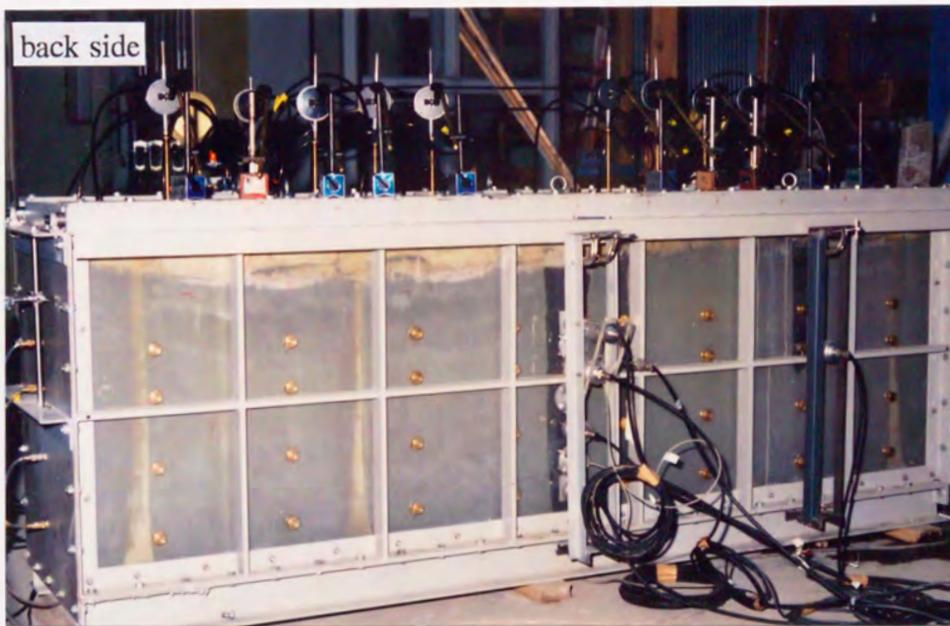
Photo. 6.7 Under preconsolidation of clay layer
