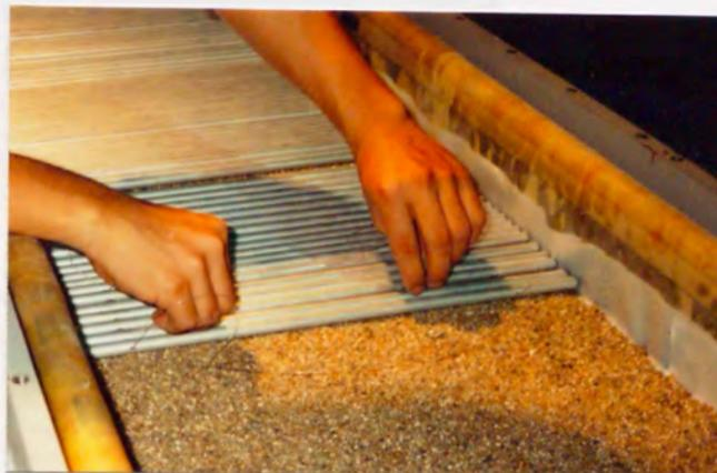
Photo. 6.6 Drainage layer, filter paper and sand layer, and aluminum pipes
