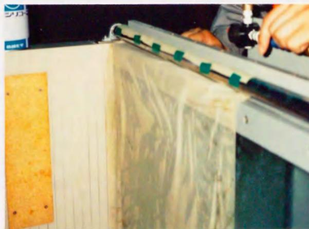
Photo. 6.3 Lubrication of side wall with silicone grease and rubber membrane
