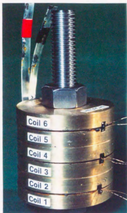
Fig.5.12 Specifications and a photograph of the Bi-2212/Ag stacked pancake coils.
