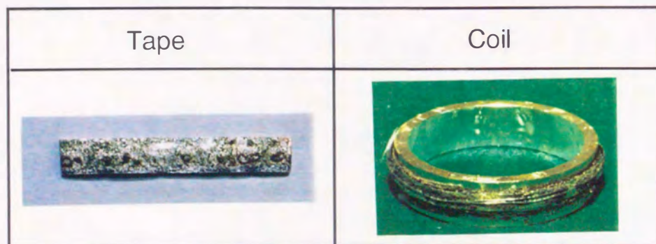
Fig. 5.4 Surface morphology for a Bi-2212/Ag tape insulated by a ceramic paper after partial melting.
