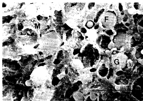
Fig. 7-2b. Microstructure of SPI-emulsion gel (control). Sample was cryofractured then fixed with glutaraldehyde and post-fixed with osmium tetroxide, as followed by vacuum drying.
