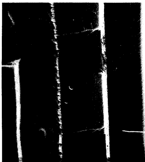
Fig. 5. SEM micrograph of slip plane in sugi (yabukuguri) wood.
