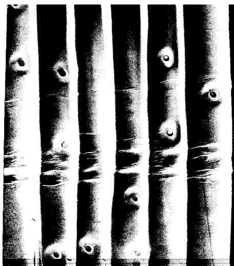
Fig. 4. SEM micrograph of microscopic compression creases in seedling sugi wood.
