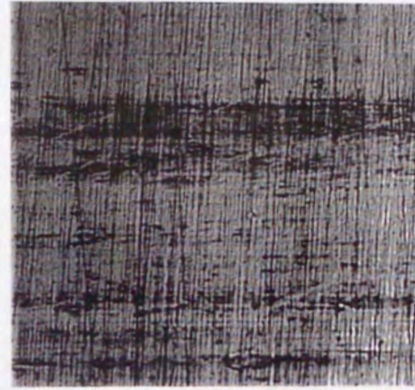
(C) UHMWPE / Stainless steel Lubricant : Ringer's solution
