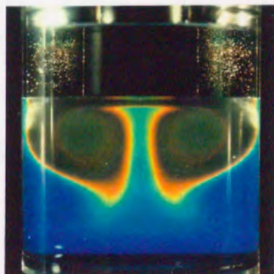
Fig. 3-15: Computed and visualized isotherms for Case (A-3). Visualized pictures were taken in two-minute intervals. Isothermal lines are at every 0.05 between -0.5 and 0.5.
