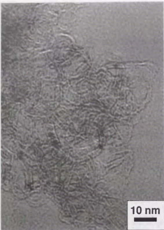
Figure 5-7 HREM micrograph of sulfided Ru-CoMo-1 / Al 2 O 3 . (a)(b) magnification under x 200K, (c) x 500K
