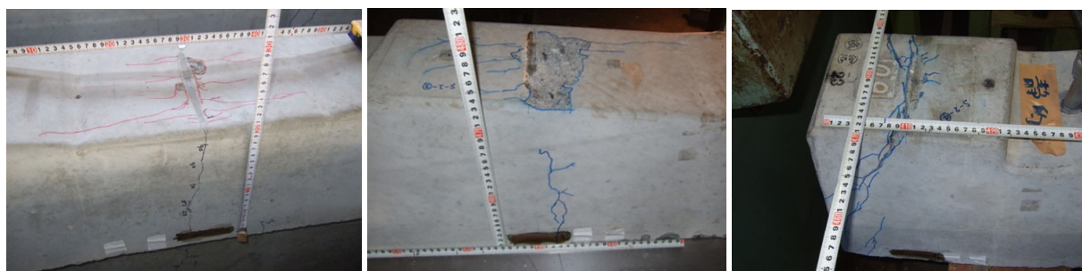
(a) S-1 (曲げ破壊)
