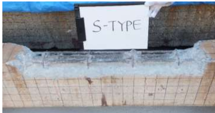
(b) S-type beam after crushed
