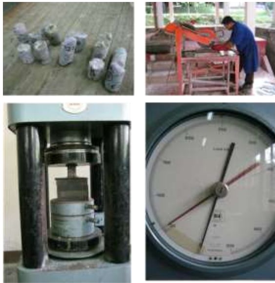
Photo 3.11 Compressive strength test
