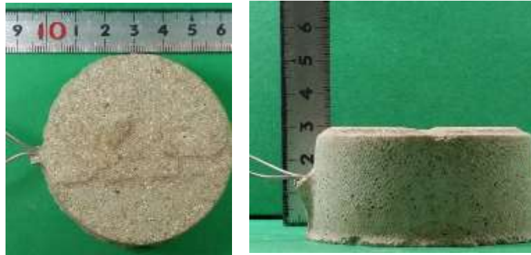
Photo 7.1 Zinc sacrificial anode XP-type
