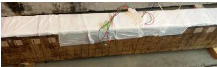
Photo 8.21 Pre-wetting before potential measurement
