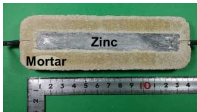
Photo 5.1 Geometry of sacrificial point anode
