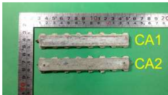
Fig 7.17 Visual observation of zinc sacrificial anode
