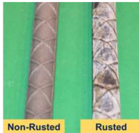
Photo 5.3 Steel bar condition before embedded
