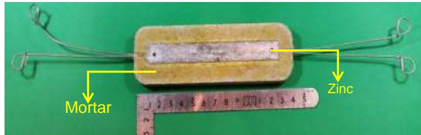
Photo 6.1 External appearance of zinc sacrificial point anode
