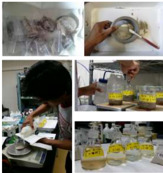
Photo 3.12 Process of chloride ion water solution
