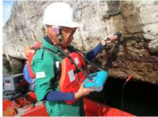
Photo 3.8 Half-cell potential measurement
