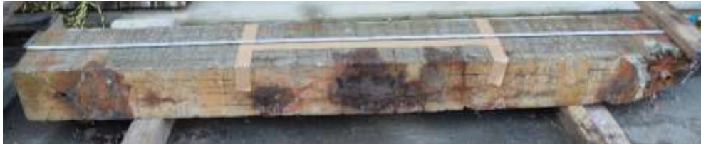
(a) Preparation of L-type beam before crushed
