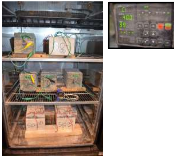
Photo 6.4 High temperature (40°C and RH 96-99%) chamber
