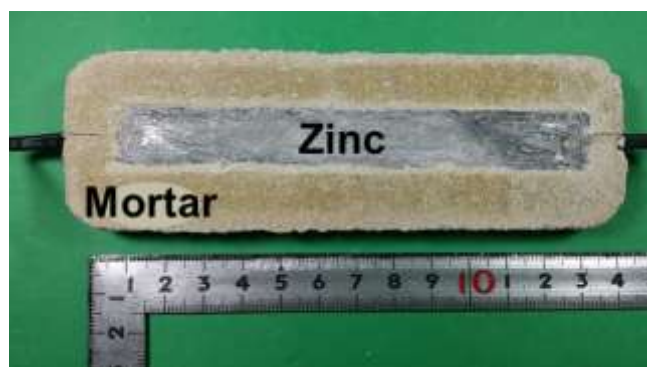
Photo 8.12 Geometry of zinc sacrificial anode F-type
