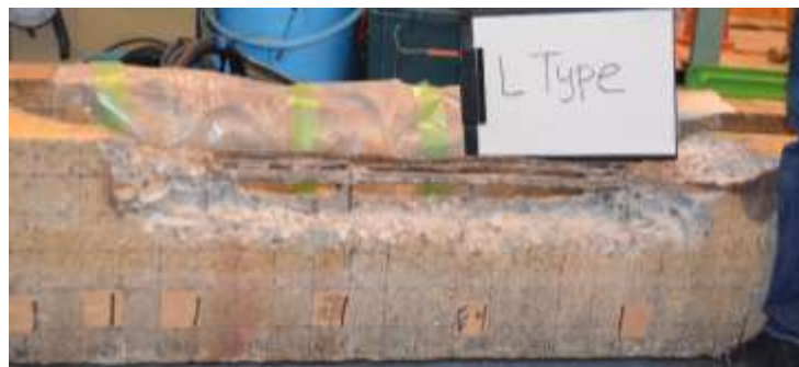
(b) Condition of L-type beam after crushed
