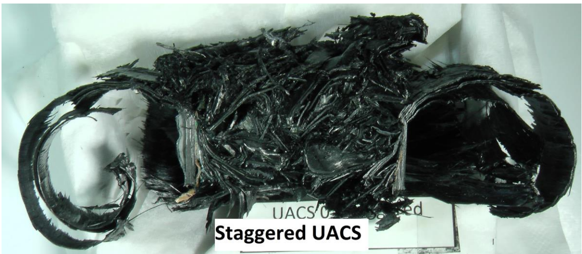
Figure 4-7: Cross-sectional view of final crushed specimen tubes.
