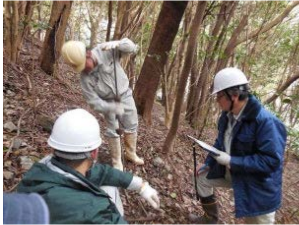
Fig. 6.5 The operation of simple penetration test
