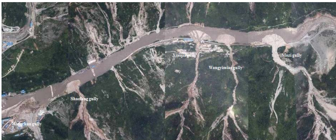
Figure 1. 1 Aerial photograph showing debris flow fans produced by rainstorm near Yingxiu town on August 14, 2010 (taken by the Ministry of Land and Resources, PRC)
