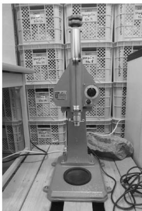
Fig.2. Photograph of the stamp mill used in this study.
