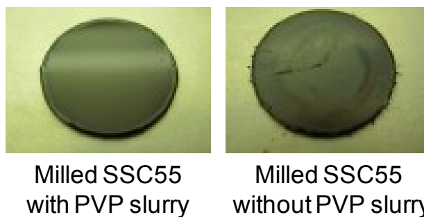
Fig. 2-4-4 Photographs of the bead-milled SSC55 slurry coated onto the electrolyte disk after drying.
