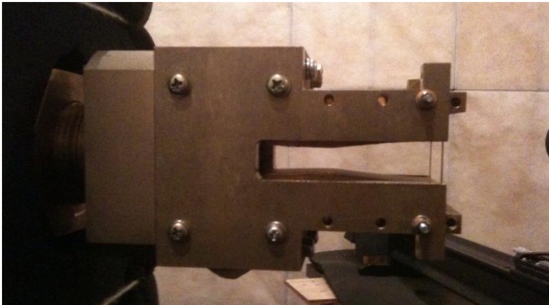
Figure 5.2 A photo of the 2-dimensional convergent-divergent nozzle
