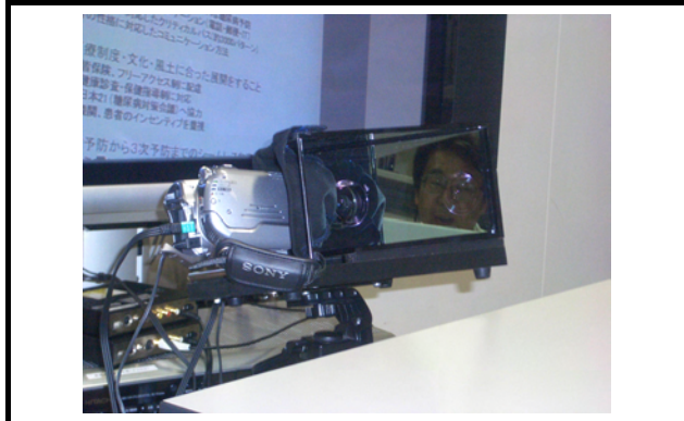
The 3D image generator combined with two DVcams
